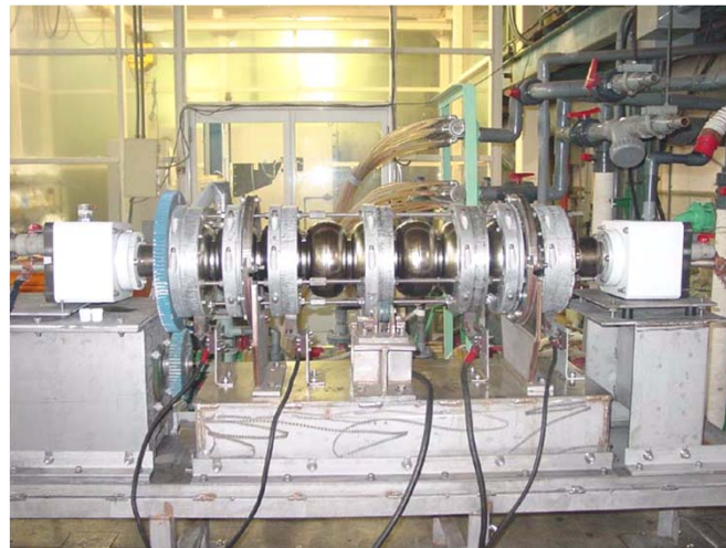
Electropolishing @Nomura Plating on May 27
