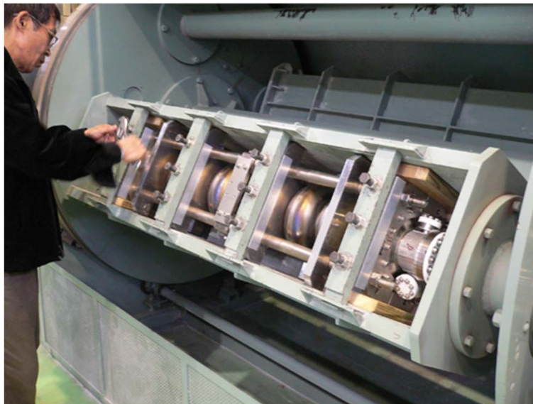
Baseline cavity No.1: Setting to CBP(Centrifugal Barrel Polishing).
